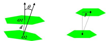
The value d is the distance between the center of the ring planes, O1 and O2. It is so chosen to represent the closest distance between two benzene rings, typically around 4.5 Å. A much larger value may run into the risk of wrongly identifying  $\pi$ - $\pi$  stacking between two benzene rings sandwiched with some other atomic species.
