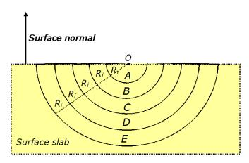
A 2D projection of a set of overlapping growing hemispheres with a common centre point, O, as defined in Option (13). Temperature values are calculated for atoms that are located in various Regions A, B, C, D and E.
