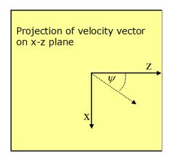
and the spreading angle,  $\psi$ . These angles are illustrated in the diagram as shown below. Consider a surface slab with the surface normal aligns along the y direction:
