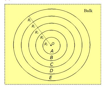
A 2D projection of a set of overlapping growing spheres with a common centre point, O, as defined in Option (13). Temperature values are calculated for atoms that are in various Regions A, B, C, D and E.
